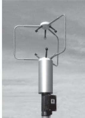
**Figure 1.** 3D sonic anemometer.
