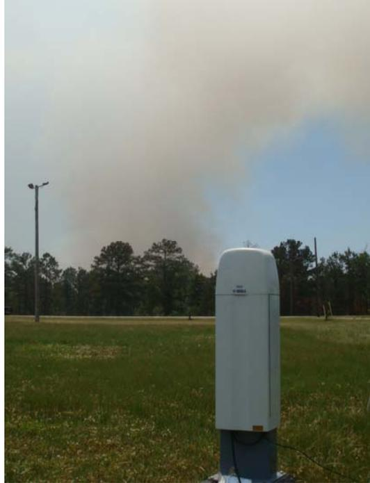
**Figure 2.** CL31 Ceilometer with smoke plume from a prescribed burn.
