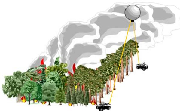
**Figure 4.** Sampling design to be used by the US EPA aerostat.
