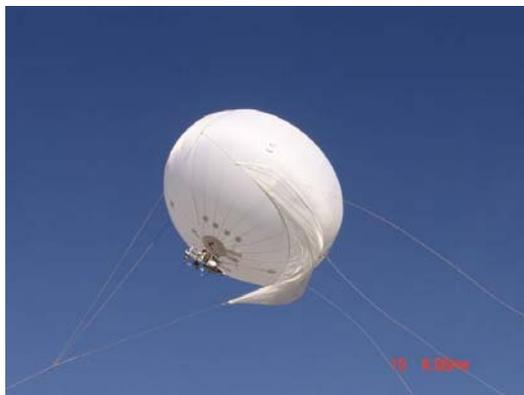
**Figure 5.** The balloon and the instrument package in operation.
